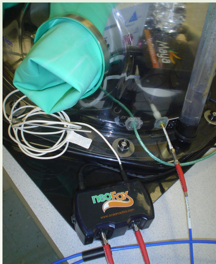
Figure 2. a. Nitrogen purge of oxygen with Mylar balloon inflated. b. Deflation of mylar balloon. c. NeoFox oxygen sensor inserted into glove box to verify oxygen levels.
